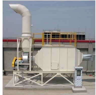
VOC Adsorption System [Activity Carbon]
