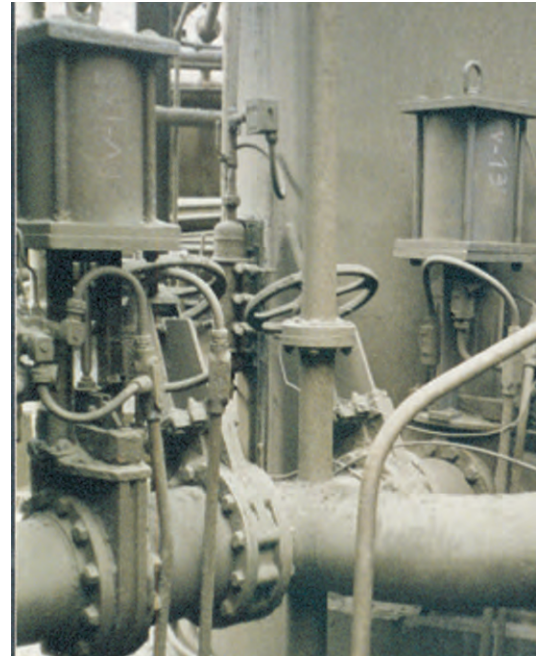
Tank isolation valve at the Andina Mine in Chile.
