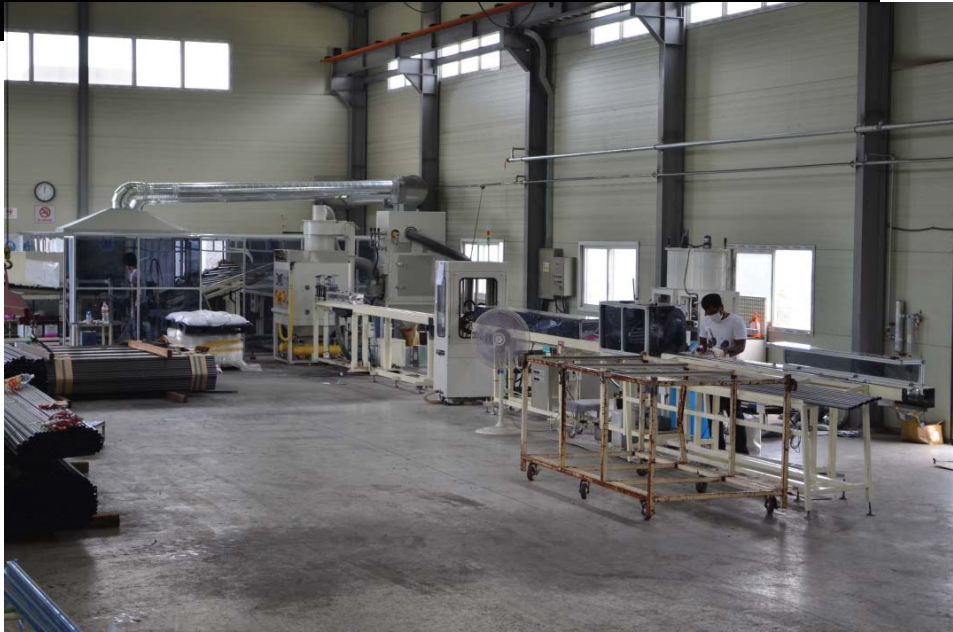
Pipe Interior-Surface Coating Line
